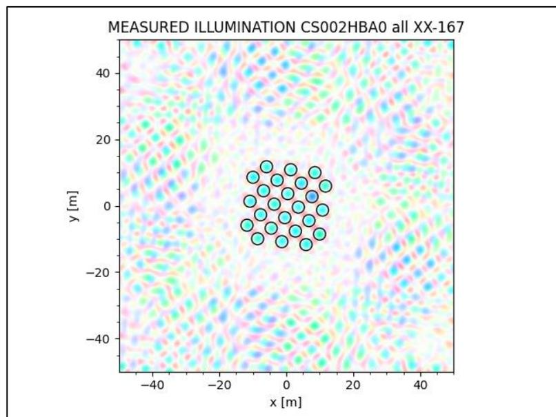
*Illumination maps for many LOFAR stations at 167.97 MHz. Brightness is amplitude, and colour is phase error. The overall state is great, and problematic antennas stand out like a sore thumb!]*
